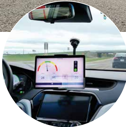
SwRI evaluated eco-driving-enabled vehicles using modeling, test tracks and dynamometers, finding that, as connected and automated vehicles are introduced in traffic, overall roadway efficiency improves, decreasing energy consumption by 15% without affecting trip time and traffic flow.
