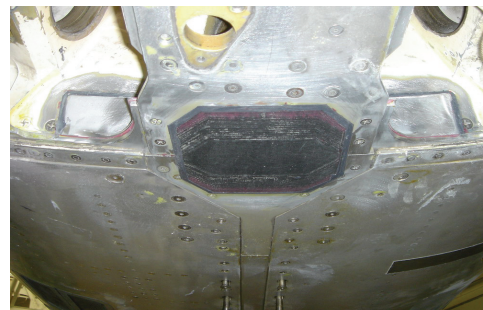
Prototype installation of F-16 bulkhead bonded repair on an in-service aircraft
