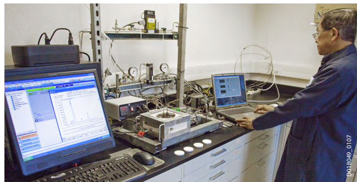
High-temperature CO 2 separation membrane evaluation system
