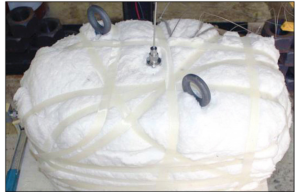
Insulated test fixture, pressurized and heated remotely from a control room during the HPHT H 2 S/CO 2 /CH 4 exposure
