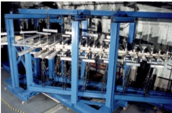
Spacious laboratories for full-scale static and fatigue tests of large structures and components; shown at left is a fatigue test of a business-class aircraft wing
