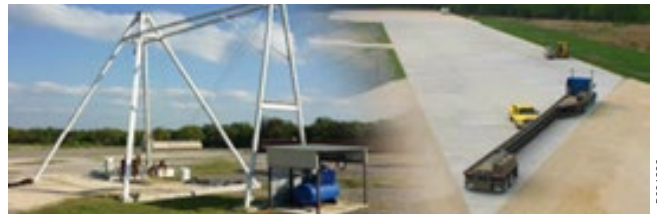
Dynamic Impact Test Facility with 600-ft x 100-ft concrete runway, large pendulum, large buried and surface-mounted reaction masses, and 30-ft drop tower to simulate various types of dynamic impact, drop and crash events
