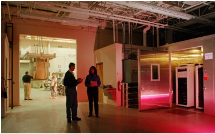
Environmental Testing Laboratory with exposure chambers and electro-magnetic and servo-hydraulic shaker tables to simulate a wide variety of transportation, storage, and operating environments including earthquake/seismic
