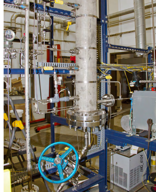
The reactor/riser is capable of processing diverse feed types such as solids, liquids, or highly viscous feeds.
