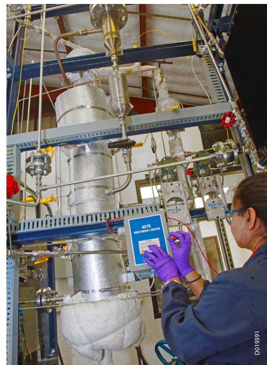
The catalyst regenerator is ignited at the start of the process.
