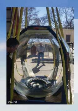
SwRI pressure tested this commercial submarine acrylic sphere in our
