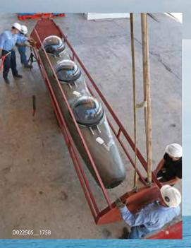
Engineers used an array of strain gauges to evaluate the pressure hull and dome windows of this deep-sea
