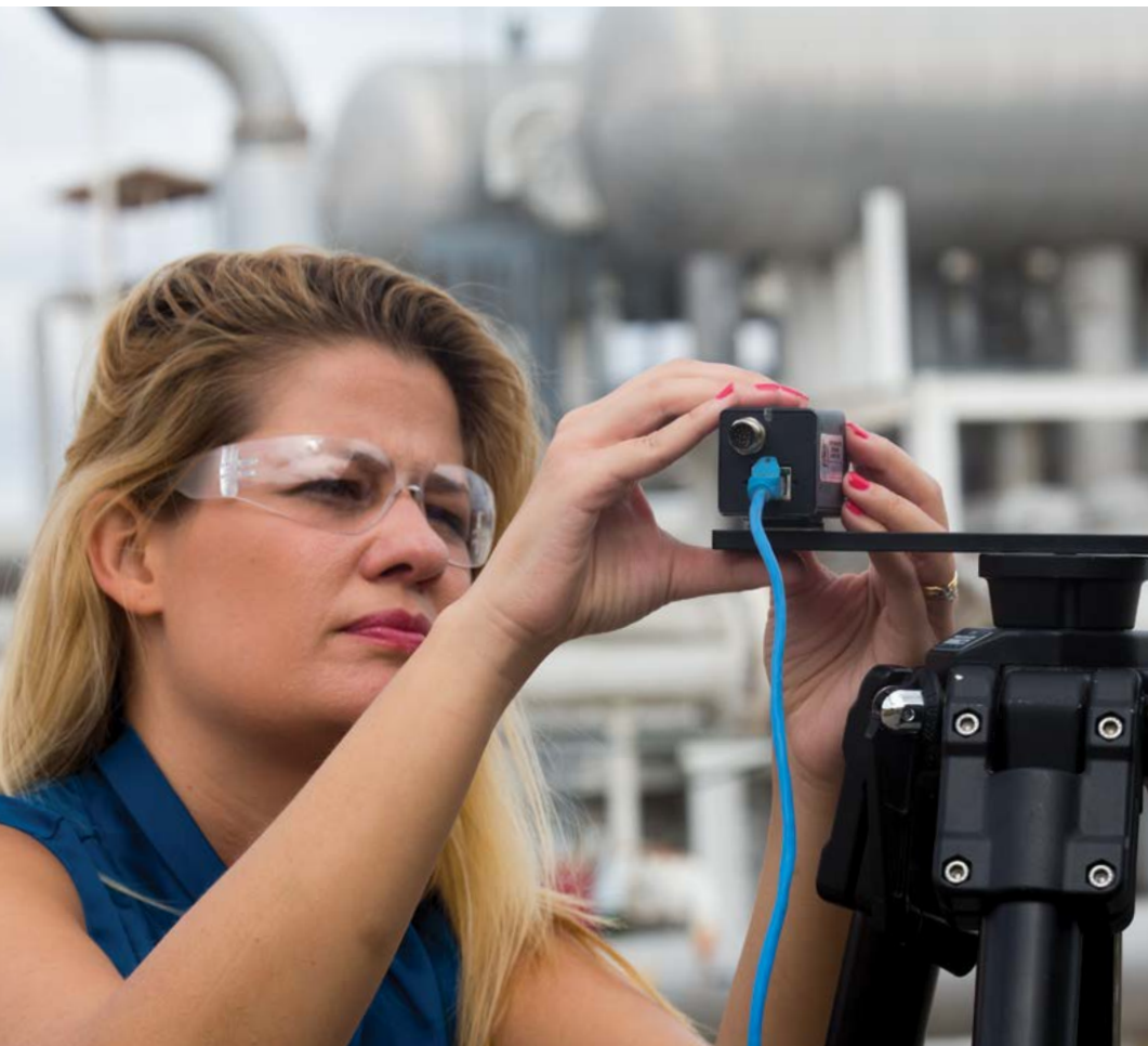
Project lead Maria Araujo sets up stationary sensors for the SLED system. Using machine learning techniques, the system analyzes sensor data to autonomously identify hydrocarbon leaks in real time.
