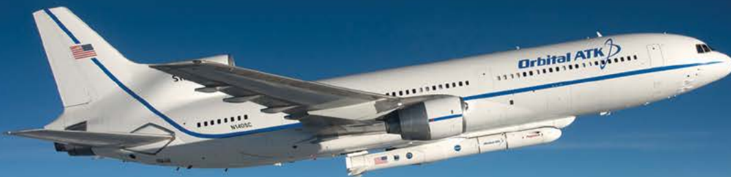
After flying to high altitude attached to the underbelly of an Orbital-ATK L-1011 Stargazer jumbo jet, the CYGNSS microsattellites were boosted into low-Earth orbit by a Pegasus XL rocket system Dec. 15, 2016.
