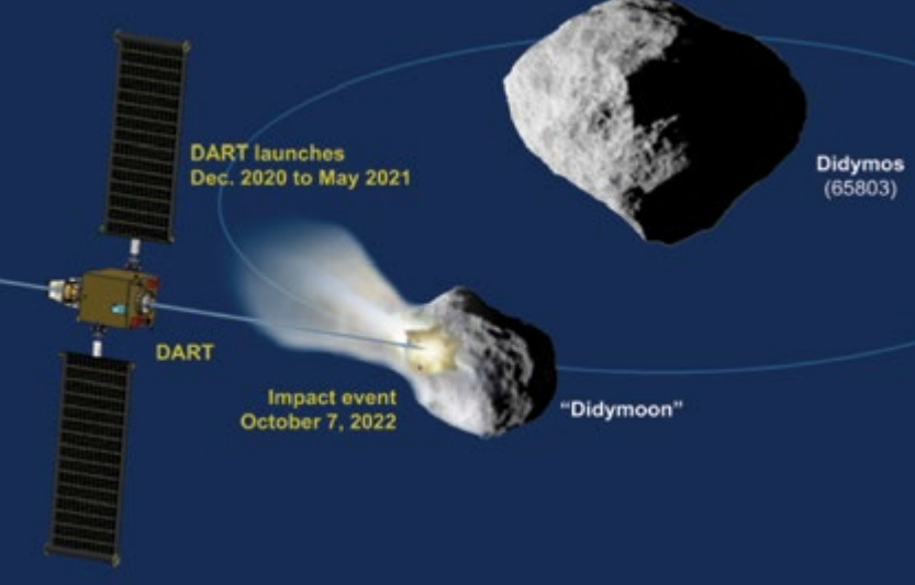
Schematic of the DART mission shows the impact on the moonlet of asteroid (65803) Didymos. Post-impact observations from Earth-based optical telescopes and planetary radar would, in turn, measure the change in the moonlet's orbit about the parent body.
