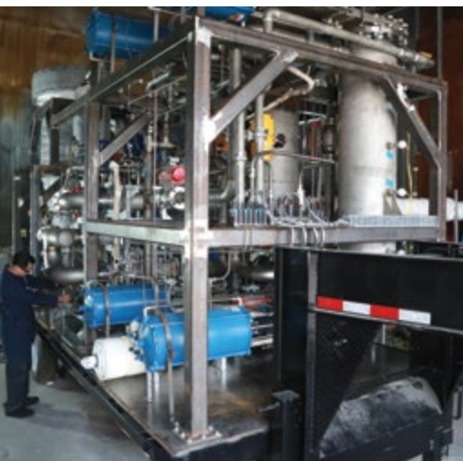
Above, SwRI's first mobile destruction system, designed to fit into a shipping container, used an engine and locally sourced soils to destroy CWA on site without producing hazardous waste.
