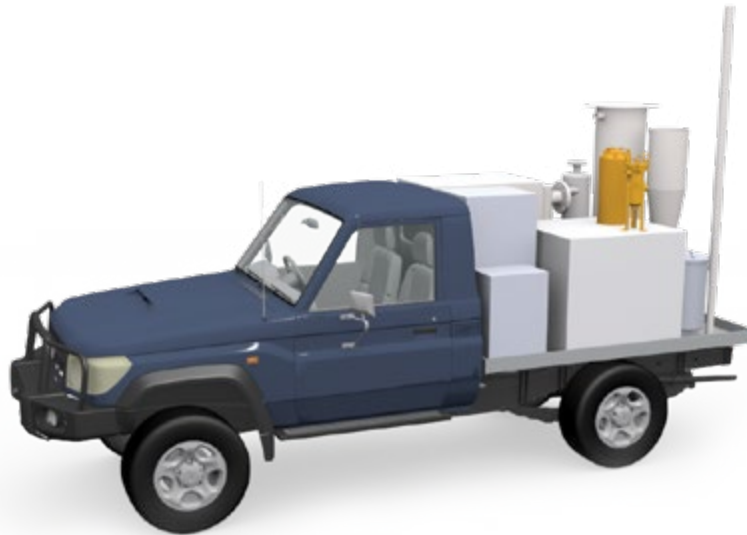
With the latest 'drive-in' design, the system can destroy approximately 10 gallons per hour at a munitions site without transport of agent or hazardous waste.
