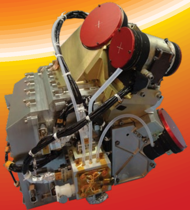
SwRI engineers worked with Caltech to build and analyze the PSP EPI-Hi instrument, designed to measure higher energy solar materials.
