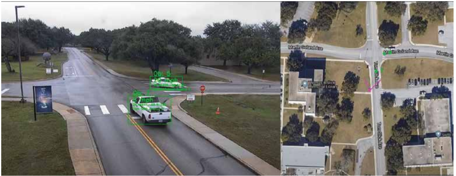
At the edge and fog level, SwRI's Active-Vision™ systems track and share trajectory information of vehicles in the vicinity using V2X.
