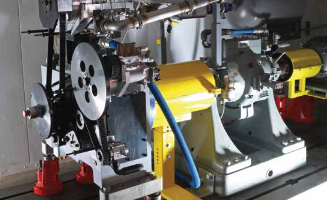
SwRI operates a medium-duty single-cylinder engine with 100% direct-injection hydrogen at 170 bar injection pressure to characterize hydrogen combustion.
