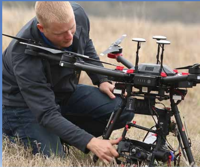
SwRI Engineer Heath Spidle prepares a drone outfitted with technology designed to autonomously detect methane leaks.
