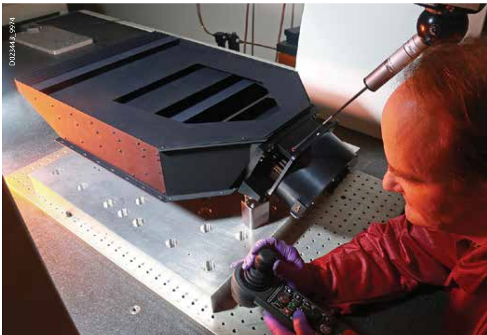
SwRI developed, prototyped and environmentally tested the Wide Field Imager using SwRI internal research funding over a period of two years. The dark baffles that form the top surface of the instrument allow the wide-angle camera to image objects over a thousand times fainter than the Milky Way.
