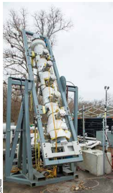
SwRI’s pilot-scale facility creates and tests natural gas foam as a safe, stable alternative to water for hydraulic fracturing, commonly known as “fracking.”
