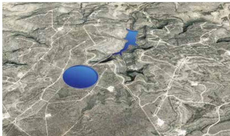
SwRI identified Indian Mesa as a potential PSH site where an upper reservoir (circle) could be built on top of the mesa and lower reservoirs could be built into the canyons below, as illustrated on this Google Earth image. In this PSH application, water is pumped to the high elevation reservoir using low-cost surplus off-peak electric power. During periods of high electrical demand, the stored water is returned to the lower reservoir, driving turbines to produce electric power when demand and prices are highest.
