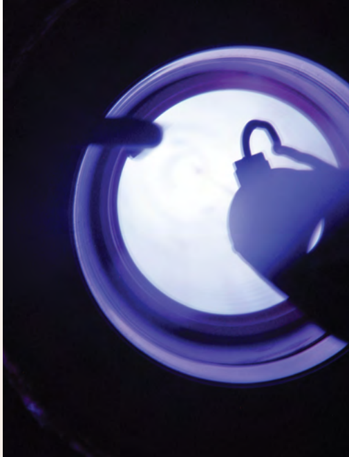
The novel process creates a plasma coating along the length of the pipe.
