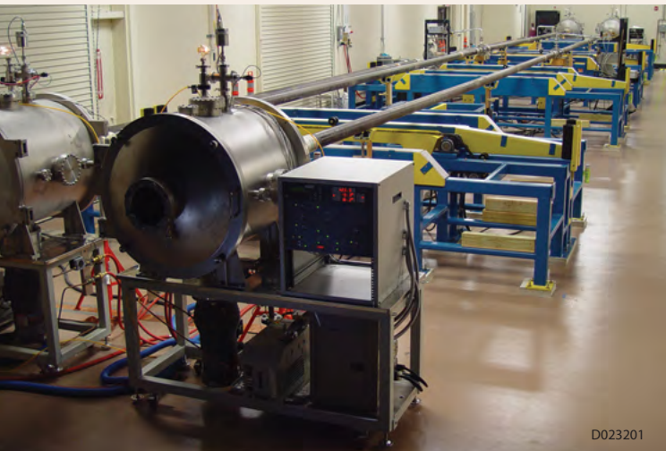
SwRI developed a vacuum process to produce superhydrophobic coatings on internal pipe surfaces. These thin, glass-like coatings are durable and repel deposits that can block oil and gas production lines.
