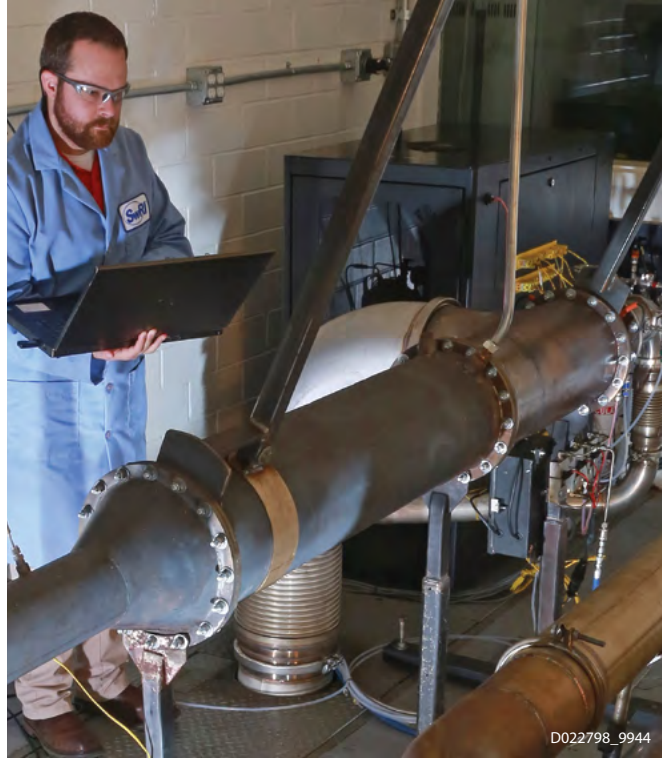
SwRI's newest ECTO-Lab system is capable of producing exhaust streams with flow rates of up to 3,250 kg/hr.
