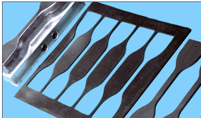
Thin polymeric and rubber specimens are 'stamped out' of flat plates with certified cutting dies for various standardized tensile specimen shapes and sizes.
