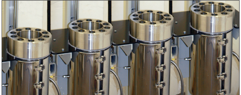
SwRI's HPHT autoclaves are used to expose different types of polymeric compounds to simulated in-service hazardous environments.
