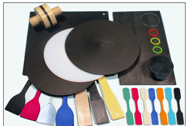
SwRI evaluates the effect of HPHT toxic gas or fluid environments on the mechanical properties of different types of polymeric compounds.
