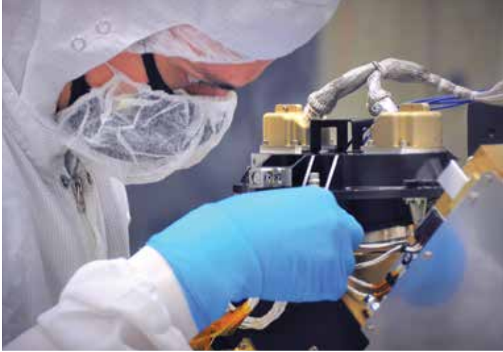
SwRI manufactured, tested and delivered the Lucy-Ralph Multispectral Visible Imaging Camera, which will take high-resolution images of Jupiter's Trojan asteroids.
