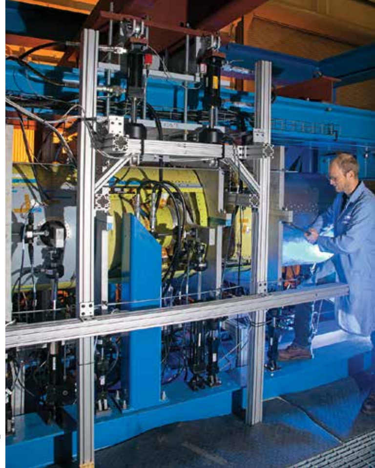
This complex custom test stand evaluates the structural integrity of Next Generation Jammer pods under real-world conditions. The pods are installed on EA-18G Growler aircraft to thwart enemy radar and targeting systems.
