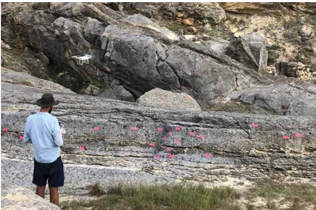
Through digital photogrammetry — reconstructing real-world objects in 3D from overlapping digital images — SwRI can extract accurate and reliable subsurface geologic information from drones flying over surface structures such as outcrops.
