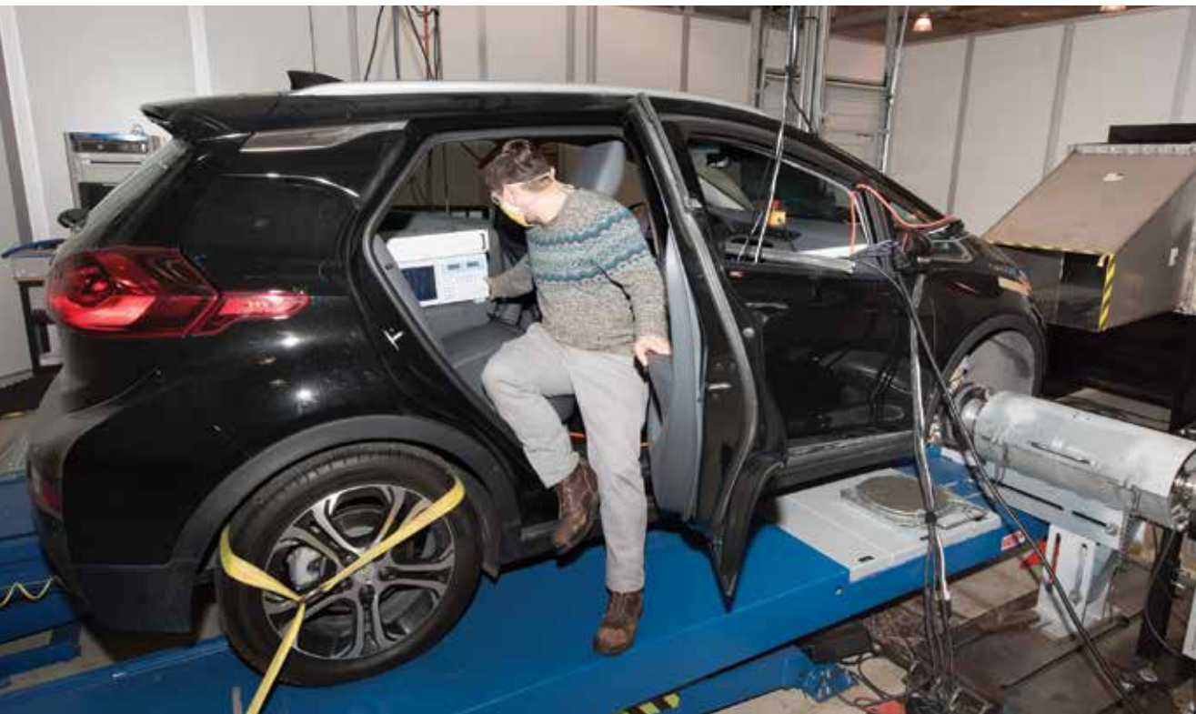
At our Ann Arbor Technical Center, SwRI is testing the efficiency of electric vehicles by measuring voltage and current throughout the powertrain while simultaneously measuring torque and speed directly at the wheel hubs.
