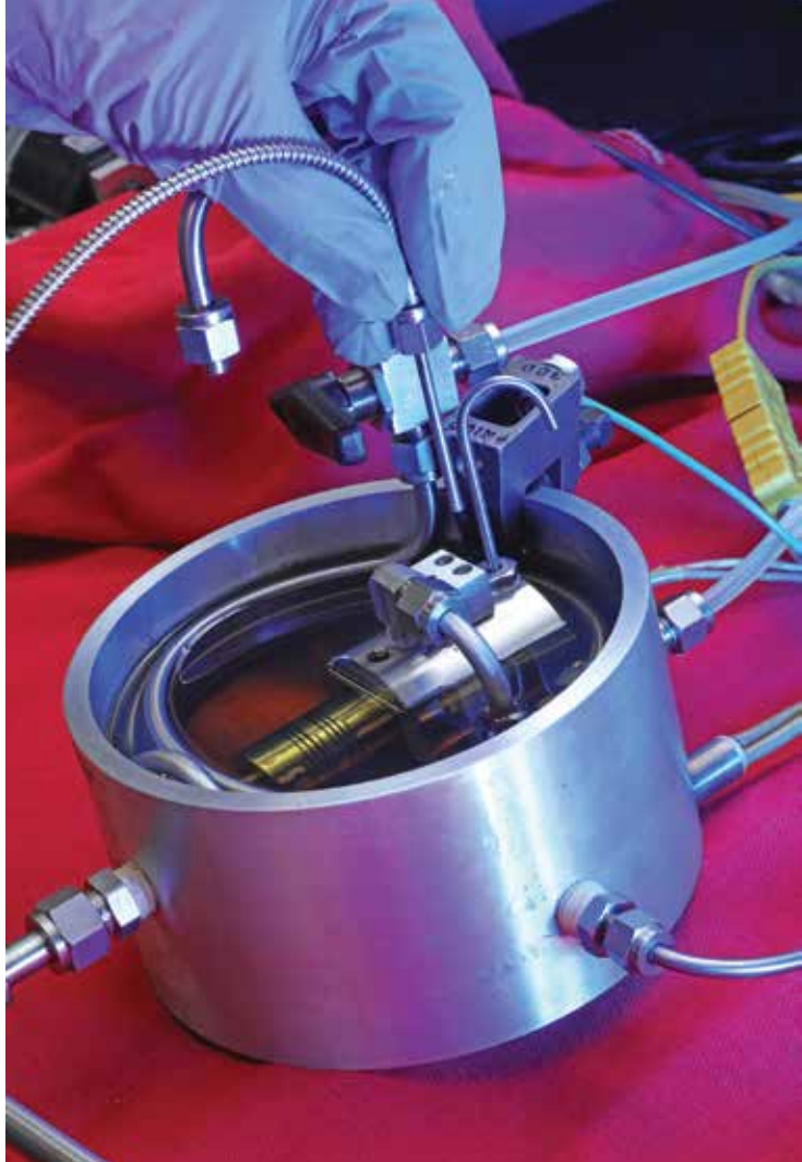
Engineers modified SwRI's bearing test rig to extend hybrid-electric testing technology from light-duty vehicles to heavy-duty trucks. The instrumentation precisely measures oil film thickness on the connecting rod bearings of heavy-duty engines.
