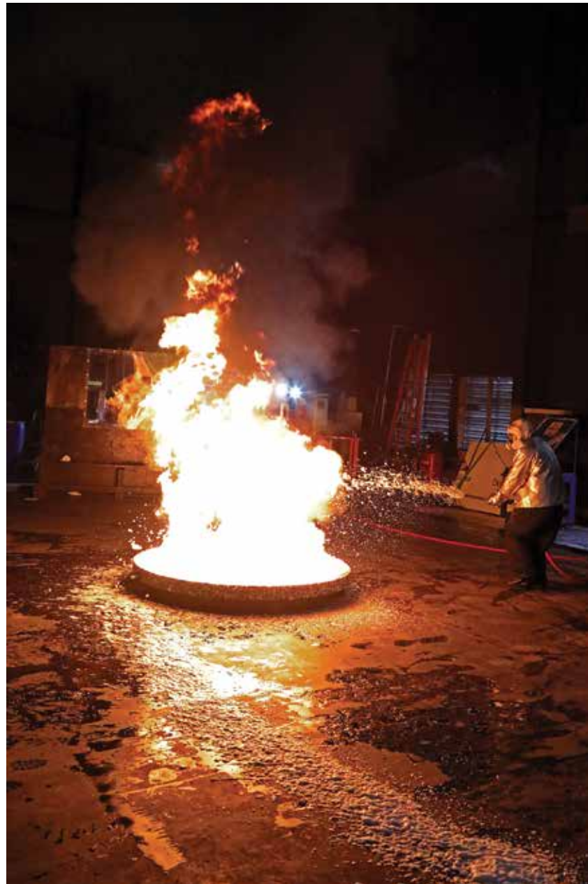
SwRI is testing a client's compressed air foam delivery equipment designed to optimize the performance of new environmentally friendly fire-suppressing foams for the military.
