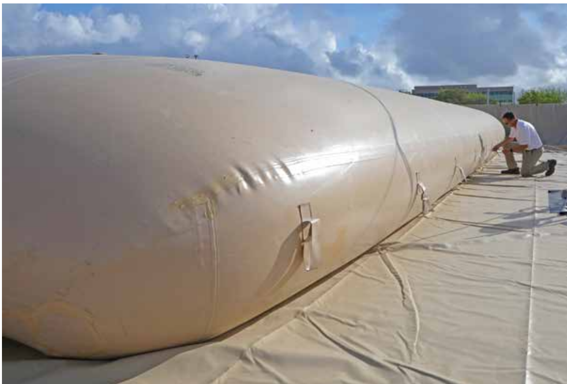
DM24639_1702c Engineers completed a fuel-bladder test facility, equipped with a concrete floor and surrounding containment structure, to test military fuel bladders. These large portable containers store fuel for battlefield operations.
