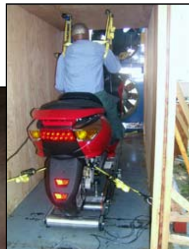
A motor scooter and anthropomorphic dummy are prepped prior to dust testing.
