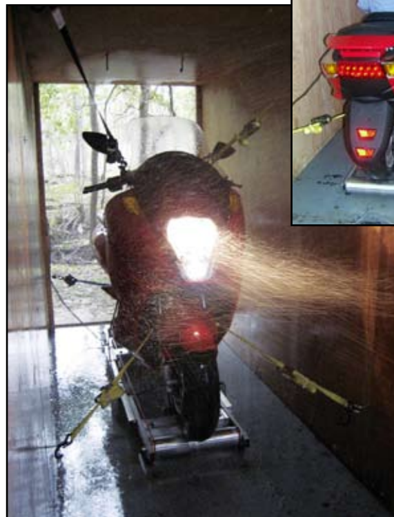
A small-scale wind tunnel is used for water spray testing of a motor scooter.
