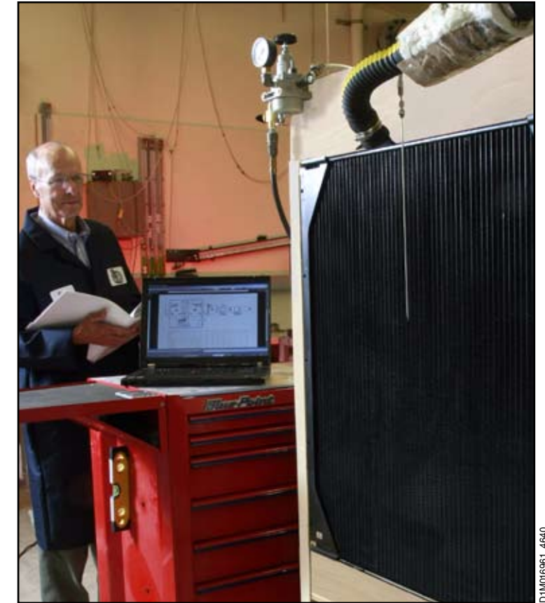
SwRI developed a new test cell to evaluate, under a variety of conditions, vehicle radiators, coolants, and related components and fluids from vehicles ranging in size from compact cars to Class 8 trucks and military vehicles.
