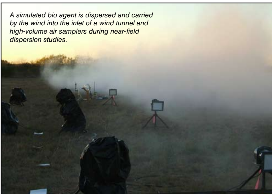
A wind tunnel, sampling probes and aerodynamic particle size analyzers are used to obtain particle size distribution data and to size specific samples for laboratory culturing during near-field dispersion testing.
