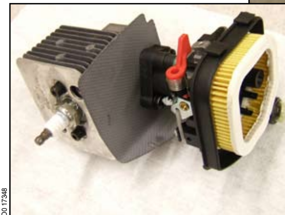
SwRI engineers measure the performance of small-engine filters such as those for lawnmowers, chain saws and string trimmers.
