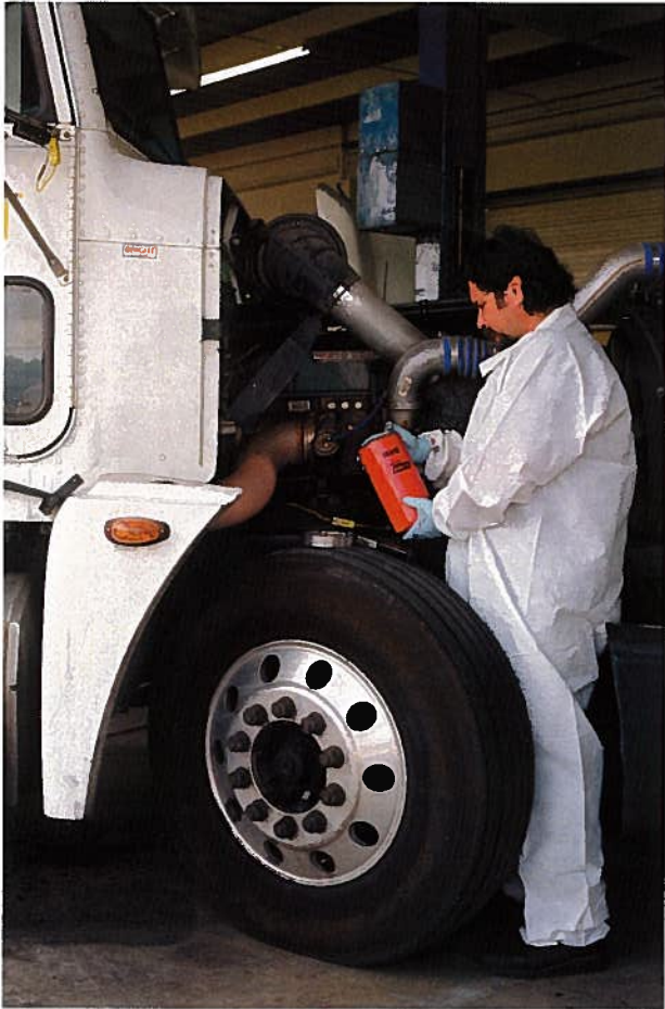
Skilled technicians perform multiple oil flushes when changing the test oil.
