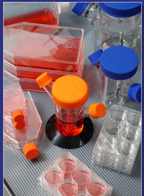
Assortment of culture vessel styles used for mammalian and nonmammalian cell growth, maintenance and amplification
