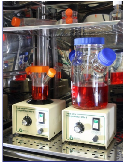
Anchorage-dependent cell culture scale-up using microcarrier cultures in spinner flasks
