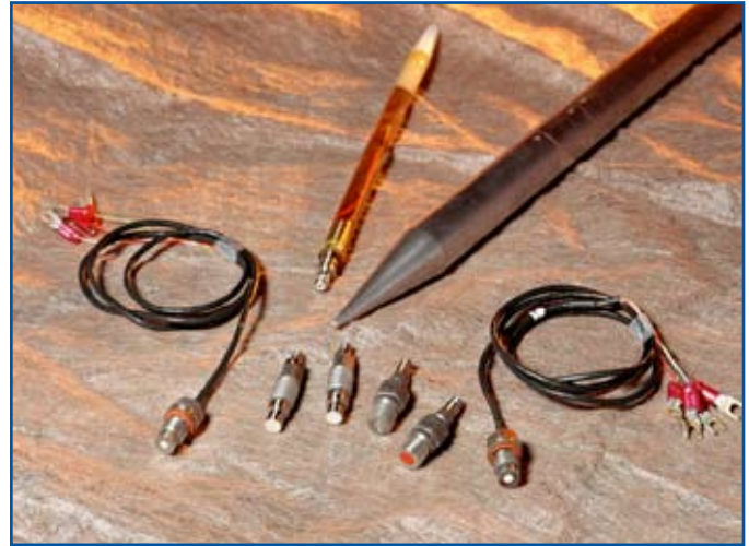
Typical piezoelectric transducers used to measure blast pressures
