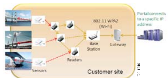
Wireless sensor network architecture
