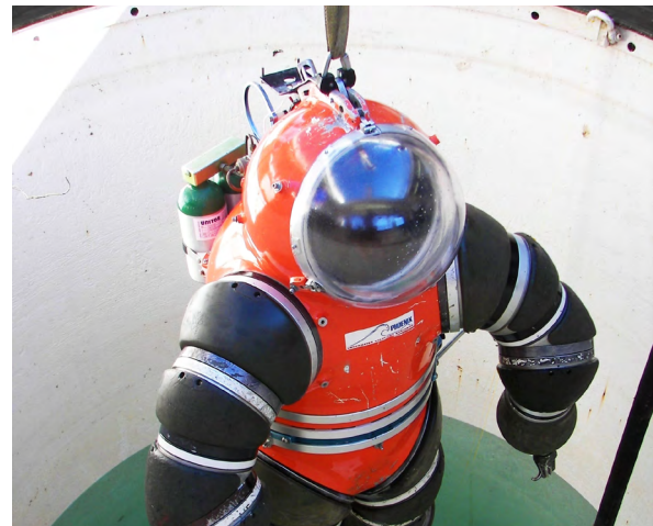
Diving suit subjected to hydrostatic pressure test
