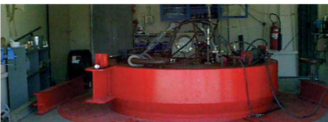
Test chamber 20 feet deep with 90-inch inside diameter
