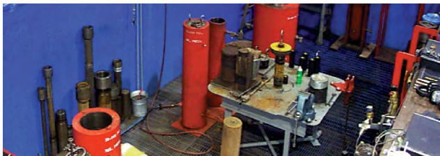
The main pressure laboratory houses more than 10 deep ocean pressure simulation chambers which are used for static, cyclic and destruct testing.
