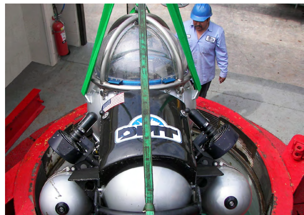
Mini-submarine being tested for ABS recertification
