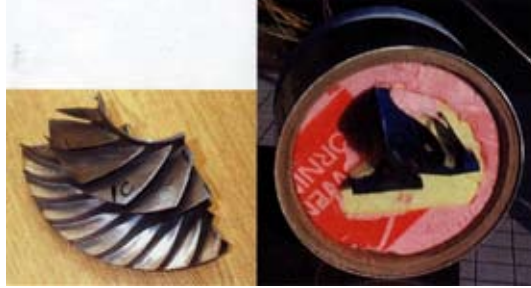
One-third of a jet engine compressor packed in a sabot for launching. Complex sabots are often needed to launch irregularly shaped projectiles.
