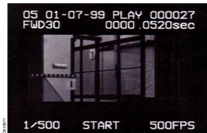
65-lb fragment-simulating projectile about to impact Lexan shield design
