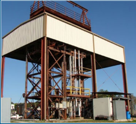
SwRI's gas blowdown facility allows for high-velocity, high-pressure-drop testing of valves, downhole tools, and other oilfield products.
