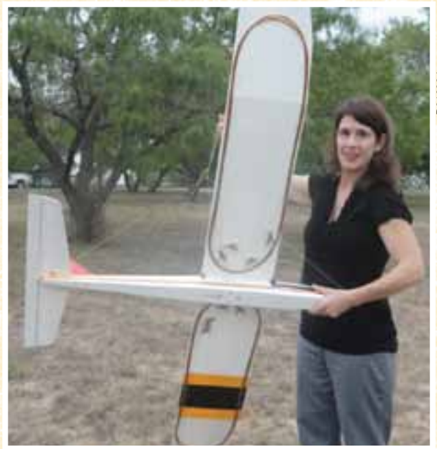
An SwRI researcher holds the Skywisp® glider prior to in situ gas collection. Capillaries are visible on the underside of the wings. The glider can be launched with a weather balloon to altitudes as high as 100,000 feet and its descent controlled to a specified GPS coordinate.
