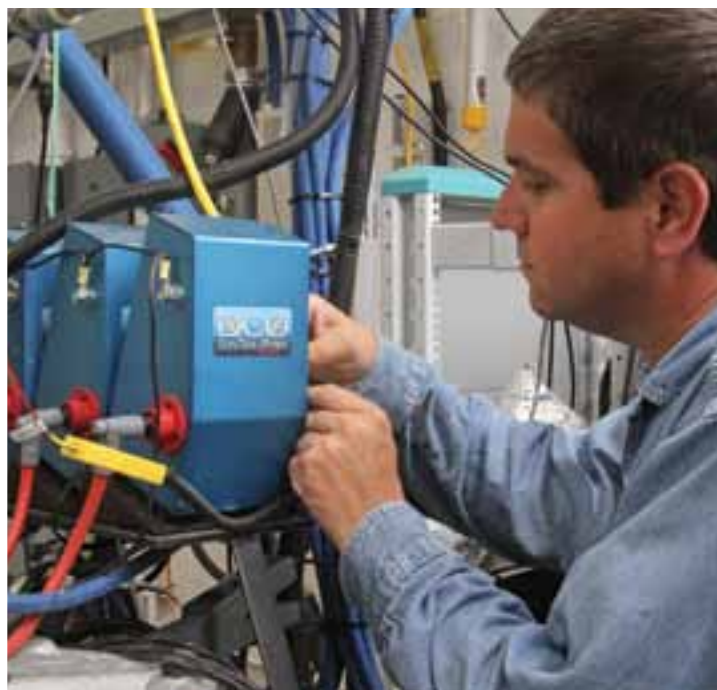
R&D Magazine named our DCO™ Ignition System one of the 100 most significant technological achievements of the past year. The novel system will allow gasoline engines to meet or exceed the efficiencies of diesel engines, but with the lower emissions of gasoline engines. This technology results in cleaner emissions, lower fuel consumption and less potential for engine "knock."
