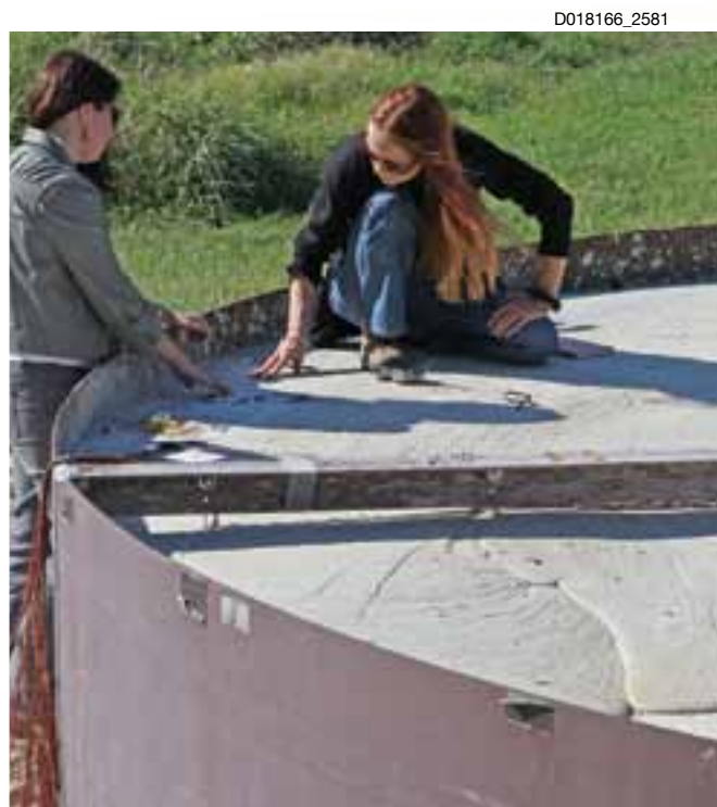
For the Nuclear Regulatory Commission, scientists conducted large-scale experiments to physically model and evaluate the performance of grout proposed to stabilize legacy radioactive wastes in tanks at nuclear material production facilities. Fissures in the grout are evaluated as potential pathways for radionuclide movement and release.
