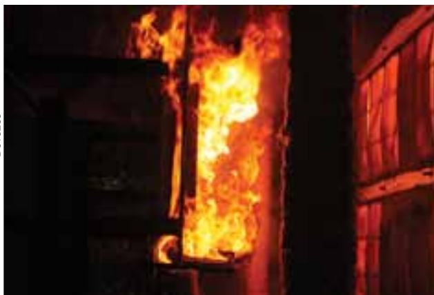
To support the nuclear power industry, SwRI built this apparatus to expose test samples to fixed amounts of radiant energy. We measure the heat release rate and amount of smoke produced to understand how components such as electrical cables perform when exposed to intense heat rather than direct flames.
