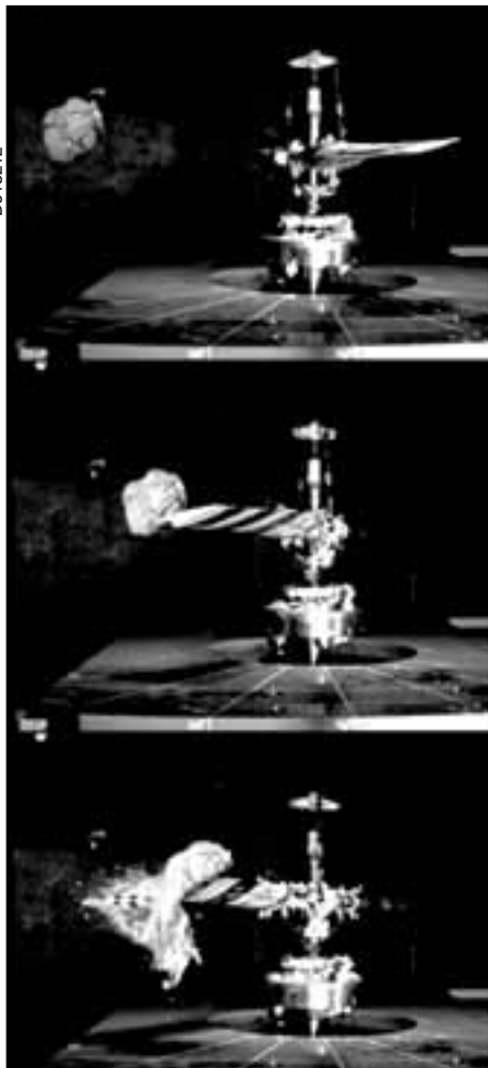
SwRI supports aircraft damage tolerance and survivability programs, conducting impact testing of stationary and rotating targets. This series shows high-speed images of a simulated bird strike on a helicopter blade ( impacteval.swri.org ).
