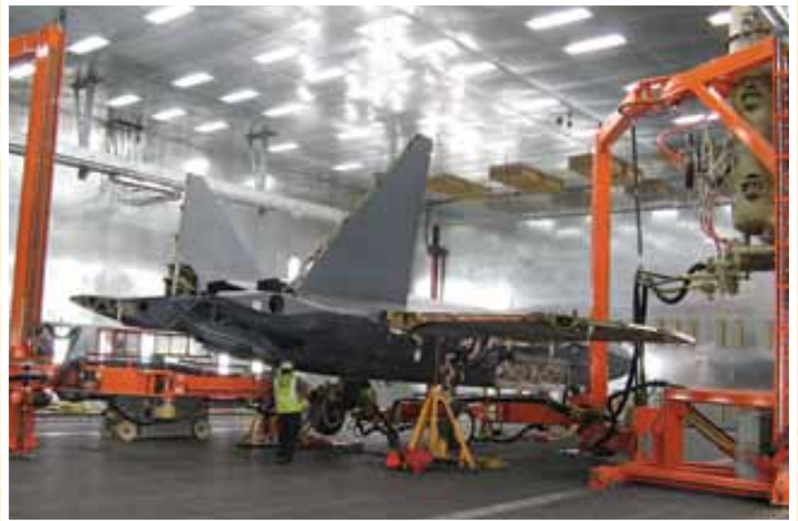
Engineers developed, delivered and installed the largest dual-robot system of its kind to depaint advanced fighter aircraft, drawing on SwRI's 25-year history in custom, large-scale robotic system design.
