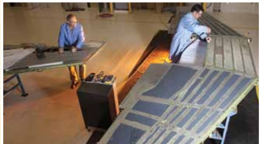
To support our aircraft structural evaluation and life extension programs, SwRI conducts destructive teardowns of high-flight-time wings removed from service to thoroughly inspect for hidden damage. Such information provides insight about wings still in service and allows aircraft maintainers to better focus future inspections and consider alternatives for repair and replacement options.
