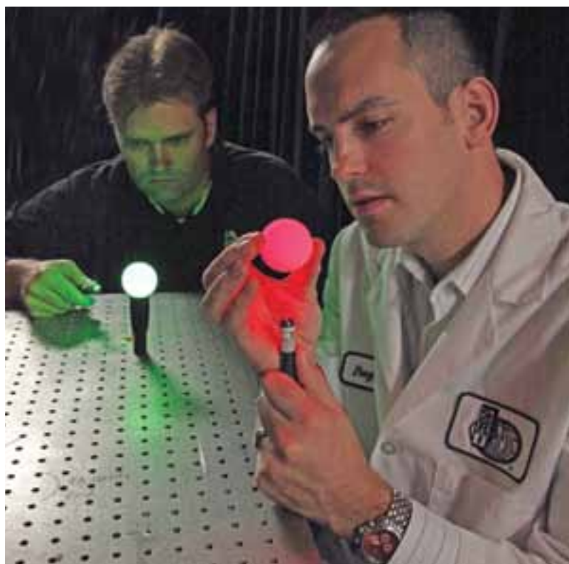
Staff members developed prototype spherically configured laser sensors to dramatically improve the performance and reduce the cost of position sensors used in a 3-D laser metrology system. The spherical sensor design is sensitive to laser light over a significantly wider range of angles than conventional cylindrical designs.
