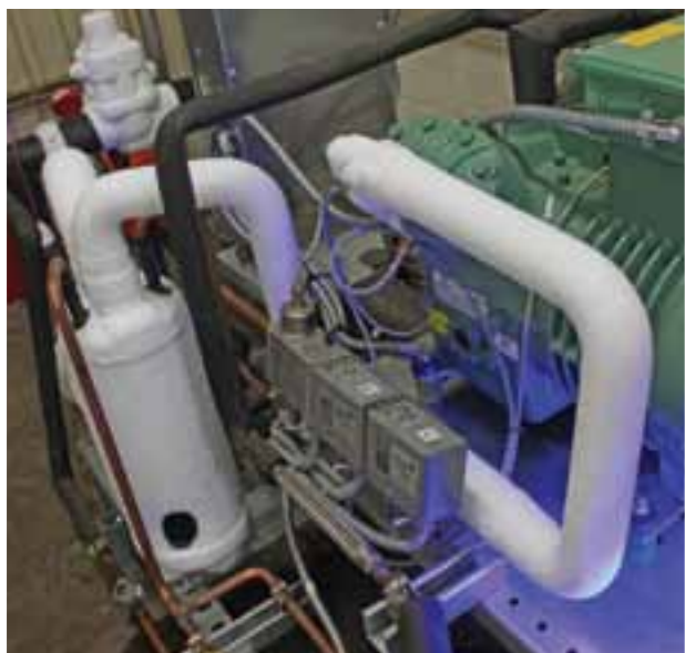
Our engineers modified a cold box to measure the time it takes oil to reach various engine components at extremely low temperatures. The test cell also evaluates flow, wear and other operating parameters at temperatures as low as minus 40 degrees Fahrenheit.
