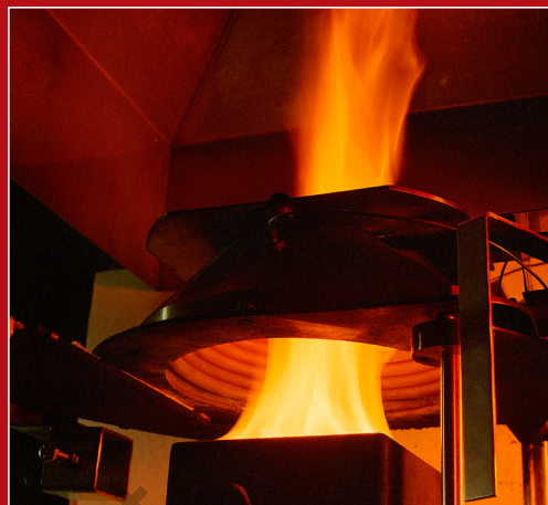
Close-up of cone calorimeter test
