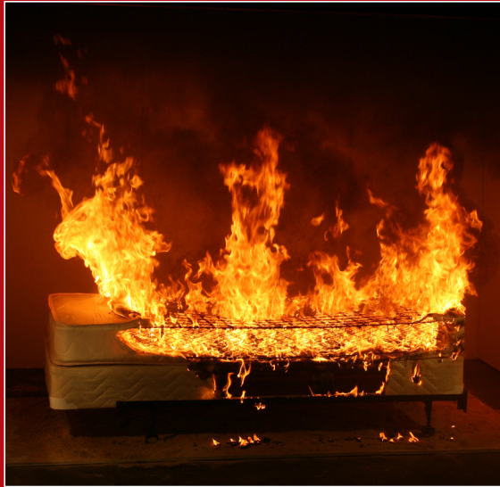
Non-compliant mattress/foundation set; peak heat release rate ~1 MW
