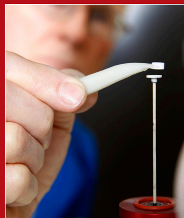
Placement of microcalorimeter test sample
