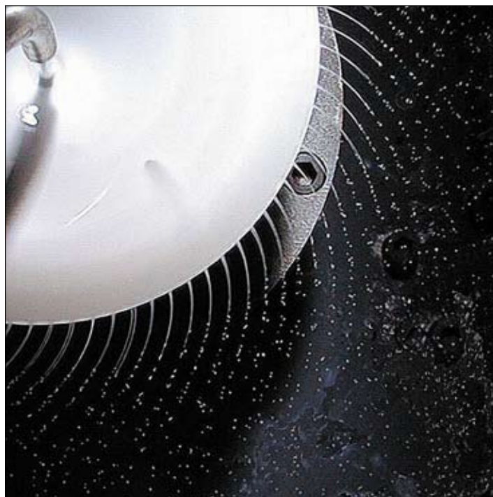
An SwRI-developed spinning disk provides spherical particles with uniform coating and narrow particle size distributions.
