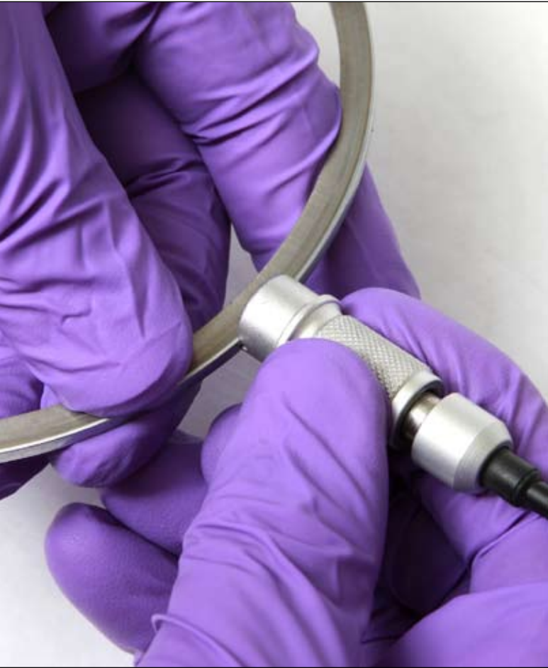
SwRI uses a Plating Surface Analyzer to ensure uniform plating thickness.
