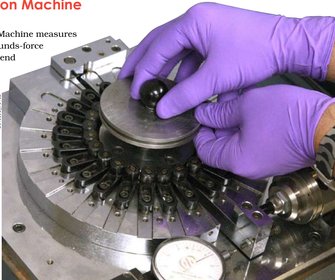
SwRI engineers use the Dorsey Ring Tension Machine to study heavy-duty diesel engine piston ring tension as it relates to engine wear and oil consumption.
