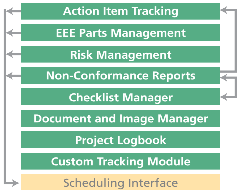
The SwRI PIMS contains nine software modules. Eight are project management modules and one is an interface module, which transfers select PIMS data to scheduling programs, such as Primavera® and MS Project.
