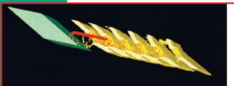
Numerical simulation of a long-rod projectile against a spaced-armor array
