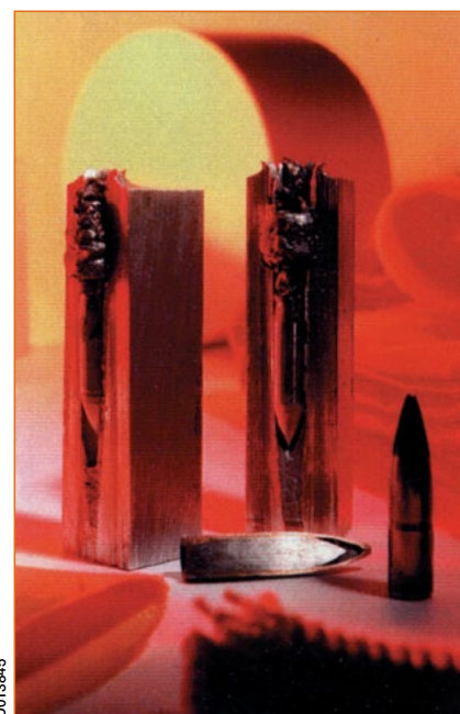
Sectioned aluminum targets after impact by a 7.62-mm APM2 bullet
