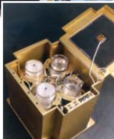
Designed and fabricated by SwRI engineers, a liquid motion experiment (top center and inset) was tested aboard the space shuttle Atlantis. The experiment investigated the motion of fluids in microgravity yielding results vital to the design of space vehicles and satellites.
