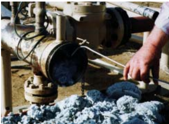
Researchers remove natural gas hydrates from a pipeline during a field test. Using the test results, Institute engineers developed hydrate remediation techniques applicable to land-based and offshore operations.
