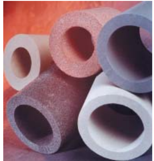
SwRI engineers used these material samples to simulate the porosity of rock in the evaluation of novel drilling fluids developed at the Institute.
