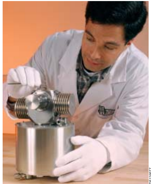
SwRI engineers designed a compression mass gauge to measure the quantity of cryogenic liquid propellants in a spacecraft tank. This gauge has proven to be more effective than conventional methods of determining liquid levels in microgravity.
