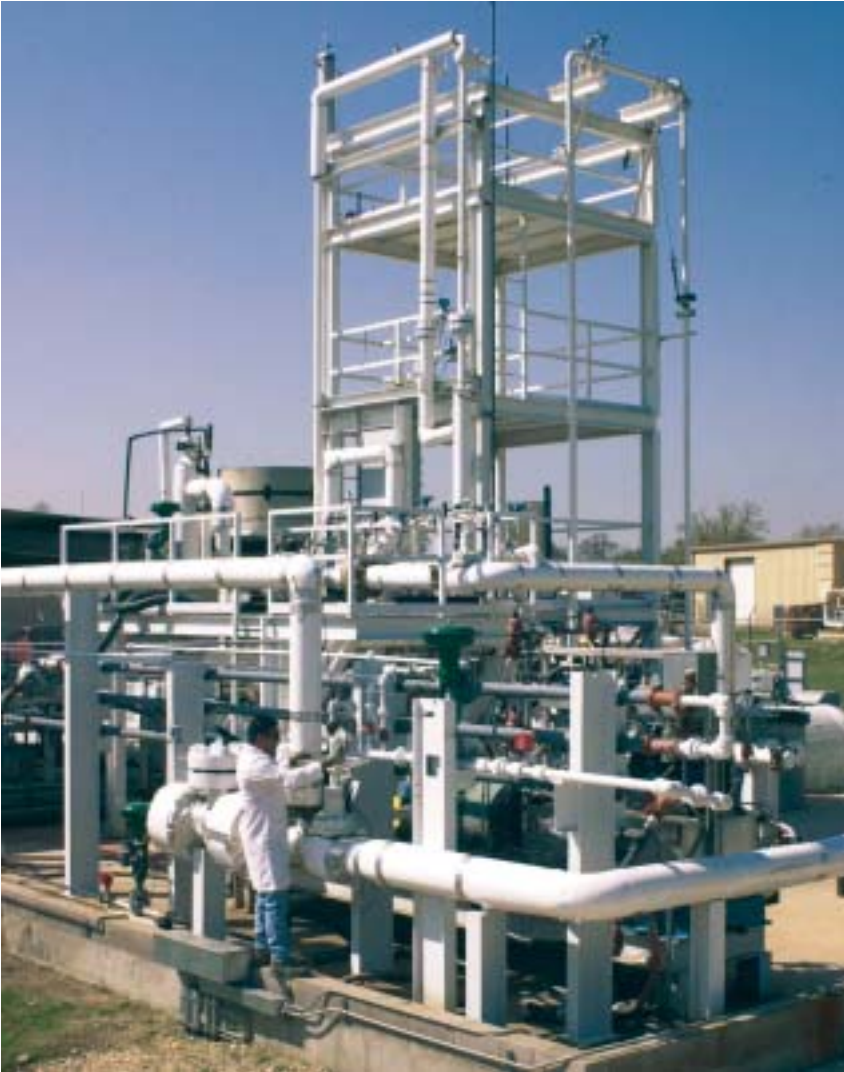
High pressure and near-freezing temperatures in deep-water environments may result in hydrate and paraffin blockages in pipelines, restricting oil and gas flow. This multiphase flow loop at SwRI is used to simulate field conditions for flow assurance studies and other multiphase flow research.
