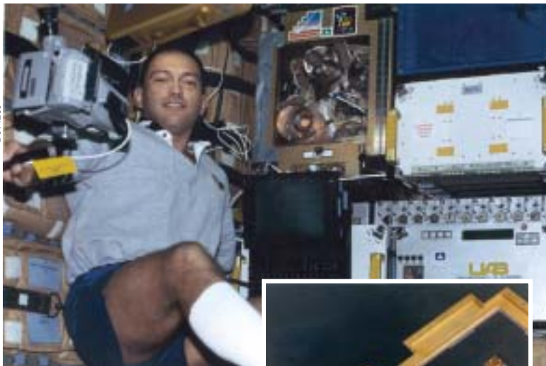
Designed and fabricated by SwRI engineers, a liquid motion experiment (top center and inset) was tested aboard the space shuttle Atlantis. The experiment investigated the motion of fluids in microgravity yielding results vital to the design of space vehicles and satellites.
