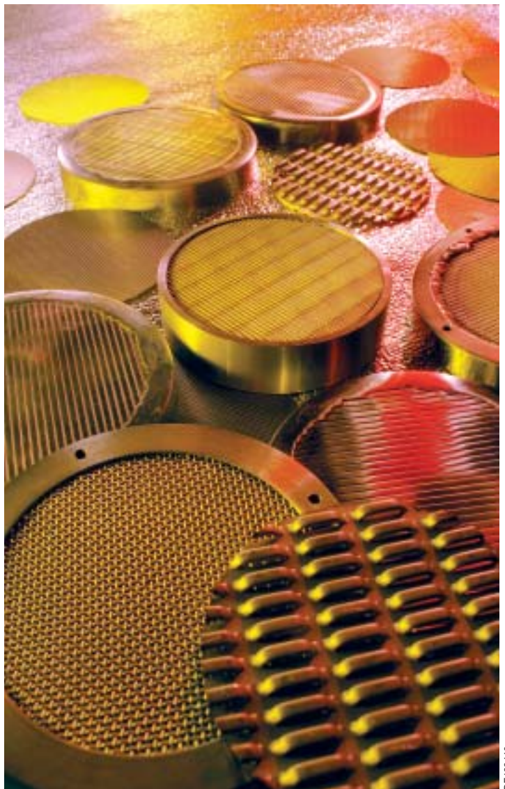
Institute-developed tests determine the erosion resistance of sand control screens used in oilfield applications. SwRI capabilities include both air-sand and water-sand systems for simulating appropriate downhole conditions.
