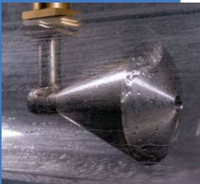
Cone meter: Testing shown under wet gas conditions
