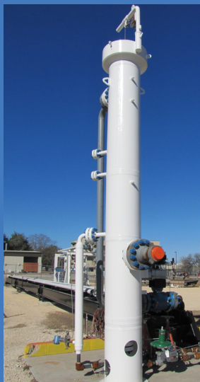
Gas-liquid separator: High-pressure performance evaluations
