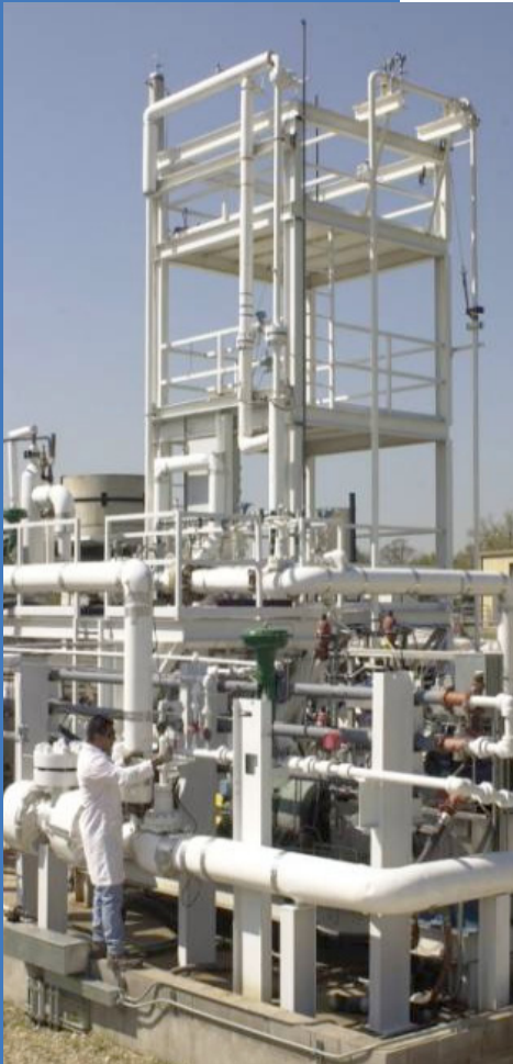
High-pressure (3,600 psig) Multiphase Flow Facility: 3-phase (oil/water/gas) field-like multiphase and wet gas conditions
