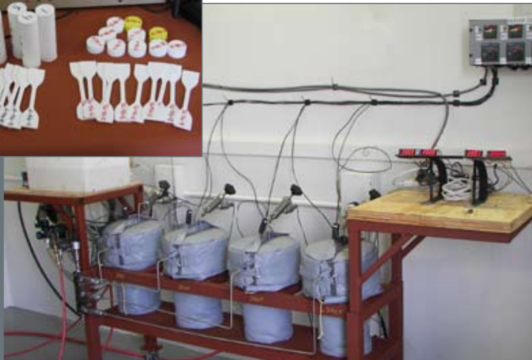
Hydroclave assembly for long-term exposure testing (Inset – Material test samples)
