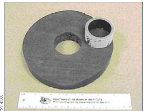
Adhesion strength test on insulation samples to evaluate bonding strength of insulation to steel substrate
