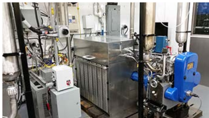
Figure 1: SwRI single-cylinder research engine with adjustable deck height feature.
