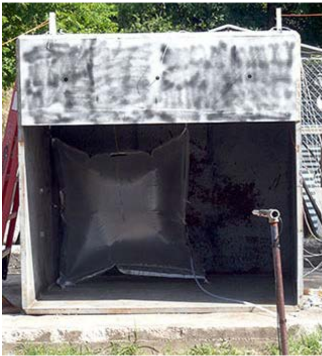
Figure 2: A bag containing a mixture of hydrogen-air within test fixture (left). Measured blast wave overpressure on back wall of structure at different sensor locations (right).
