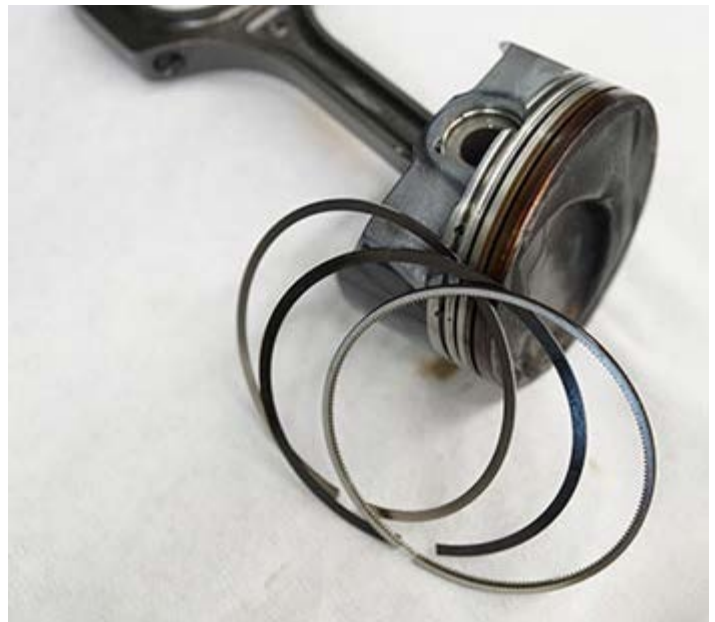
Figure 1: Engine piston rings after removal from engine
