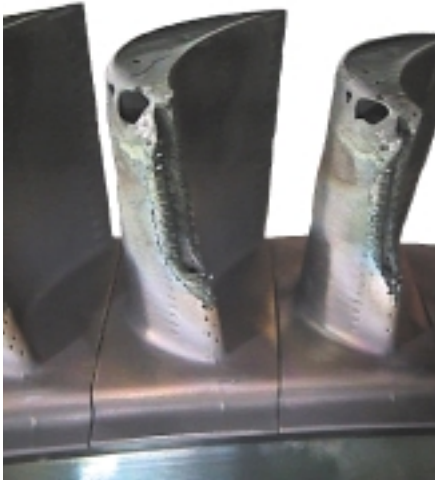
For the Air Force, our staff members analyzed turbine engine performance data. This resulted in development of training and technical manuals that assist with the detection of impending aircraft engine problems, such as the wear in the turbine blade shown.
