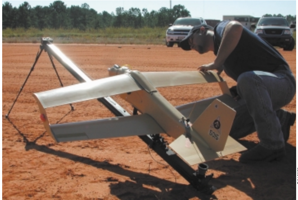
Since 1993, SwRI has performed a lead role in developing automated flight control systems for small-scale unmanned aerial systems and unmanned aerial vehicles, such as the Buster system shown.
