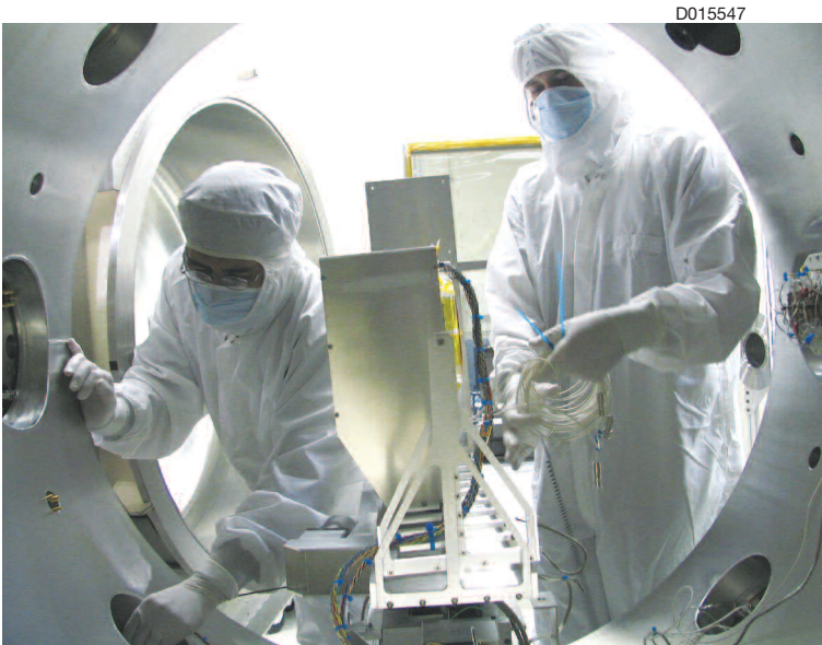
In cooperation with Los Alamos National Laboratory, SwRI is building the IBEX Hi instrument. Here, the engineering model is prepared for testing in an SwRI vacuum calibration chamber. SwRI leads the IBEX mission to study the interstellar boundary.
