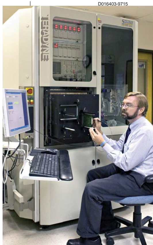
Staff members updated an existing Air Force tester to replace an outdated test system for AIM-9 missile interface components used on the A-10 aircraft. We developed test requirements, test program sets, and interface test adapters and provided system integration and testing. The new system reduces lifecycle maintenance costs for the aircraft.
