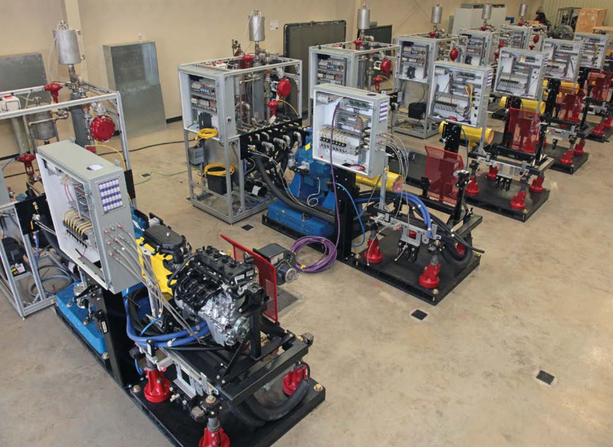
SwRI designed and built six identical test stands to support development of the new Sequence IVB engine oil test for the lubricant industry. The test stands are designed to operate a 1.5-liter gasoline engine with a 250-horsepower eddy current dynamometer.
