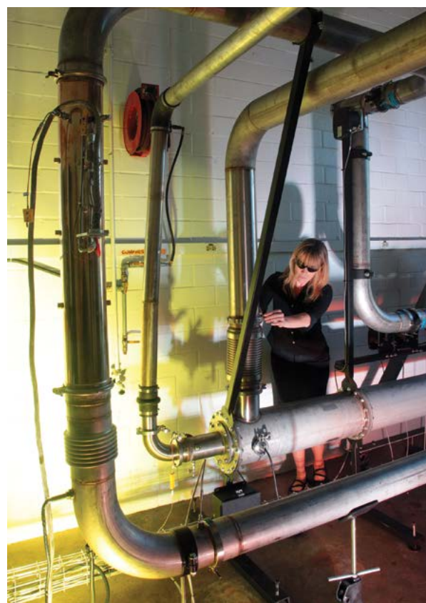
Our Hot Gas Transient Reactor (HGTR®), developed using internal funding, simulates diesel engine exhaust. The HGTR system allows researchers to evaluate catalysts without using an engine.
