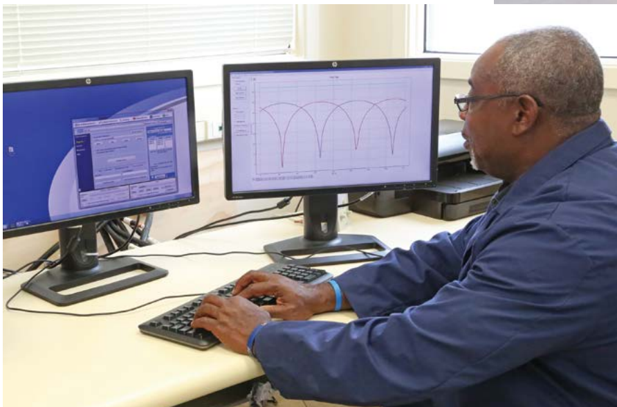
Our Rotary Test Facility includes a six-meter turntable (above) to evaluate antenna assemblies. Recent additions to the facility include a permanent control room building (above, in background) with new hardware and software that measure and display antenna patterns quickly and easily (left).
