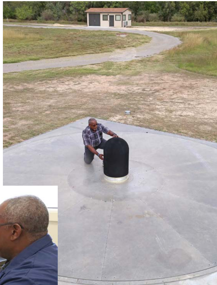
Our Rotary Test Facility includes a six-meter turntable (above) to evaluate antenna assemblies. Recent additions to the facility include a permanent control room building (above, in background) with new hardware and software that measure and display antenna patterns quickly and easily (left).
