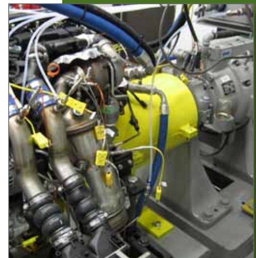
Light-duty diesel test cell installation
