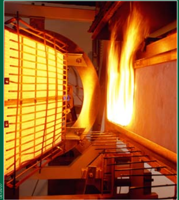
Flame spread testing per Part 5 of Annex 1 of the IMO FTP Code
