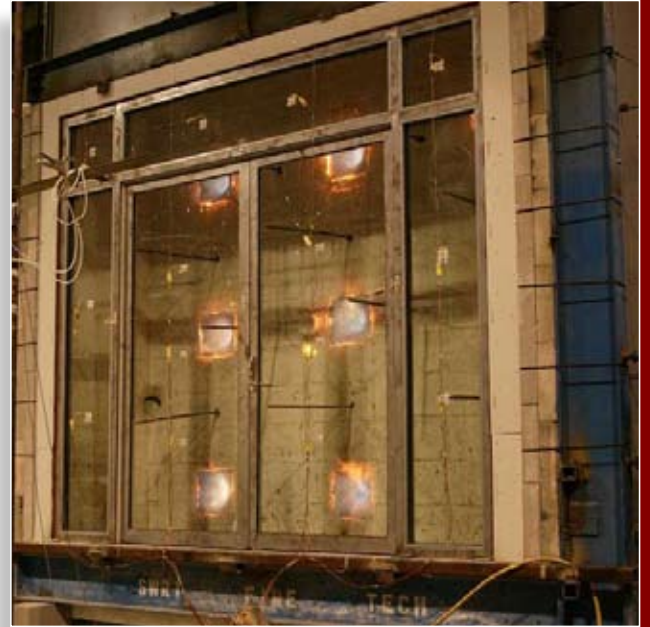
Glass wall and double door assembly being tested on SwRI's large-vertical furnace
