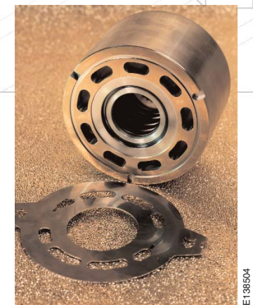
SwRI engineers optimize the valve plate interface of a motor and pump to meet industry or client requirements for noise, stability, leakage, and durability.
