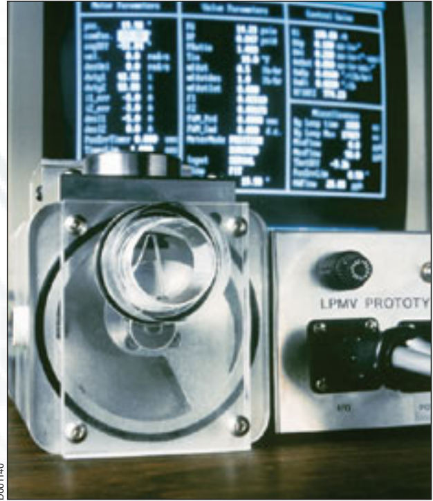
Experienced engineers develop experimental equipment to provide proof-of-concept for innovative systems. SwRI designed and built this smart, low-pressure, natural gas metering valve to meet the fuel control needs of large, stationary, alternate-fueled engines.
