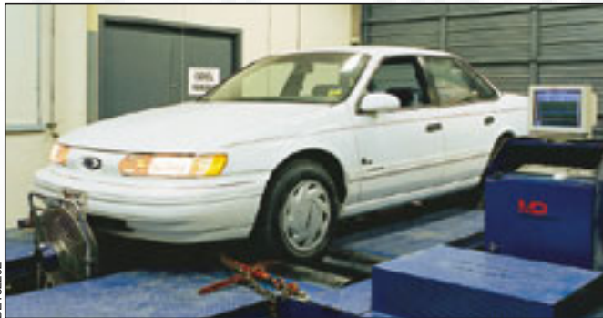
Systems developed in the test cell are often refined in a vehicle. Engineers use compact RPECS versions to evaluate production-intent vehicles in post-test cell development.
