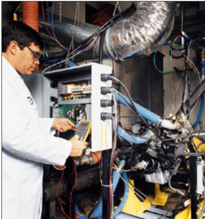
The SwRI-developed RPECS, used extensively in test cell developmental applications, is easy to modify and troubleshoot.
