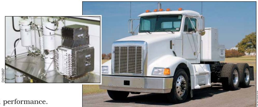
As part of the SwRI fuel cell integration activities, engineers are developing a fuel cell-powered electric drive system for a Class 8 tractor. The inset illustrates a laboratory setup for a fuel cell-powered auxiliary power unit.
