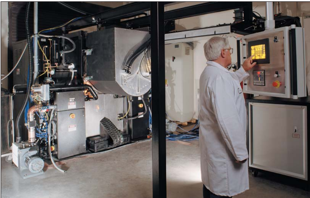
SwRI developed a pilot-scale manufacturing system for catalyzing practical quantities of PEM fuel cell electrode material under a Department of Energy-sponsored program.
