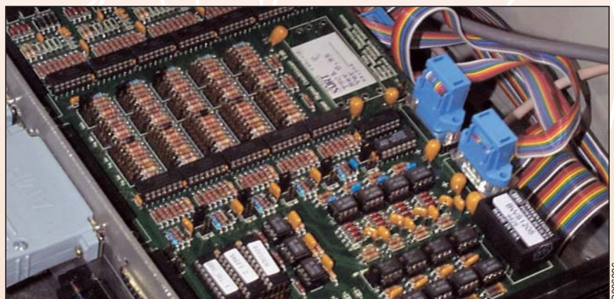
An SwRI-developed vehicle controller operates this vehicle as a “flex-fuel” system, using advanced model-based algorithms to control the engine and transmission based on different fuel types.
