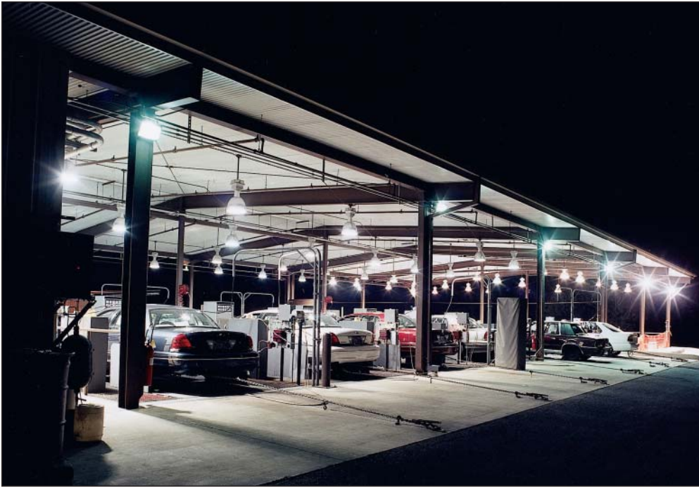
Vehicles on the mileage accumulation dynamometers are run at speeds up to 100 miles per hour. The SwRI mileage accumulation dynamometer facility provides rapid, cost-effective vehicle testing.
