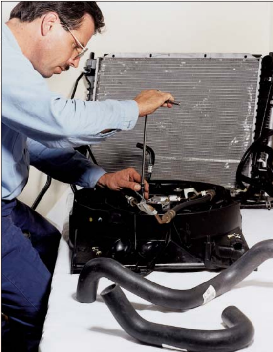
SwRI staff members, with extensive experience in automotive and vehicle heat flow, modify automotive cooling systems to accommodate higher powertrain capacity.
