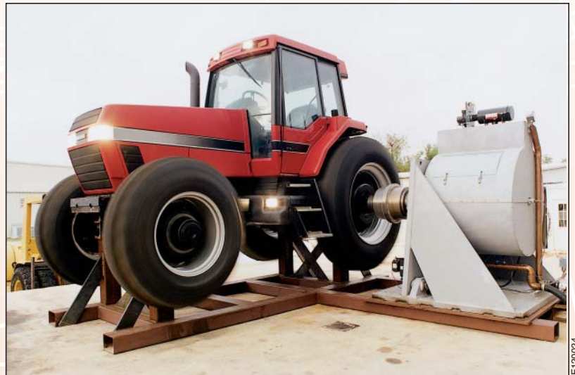
SwRI conducts high-torque, low-speed testing of agricultural, construction, and off-road equipment to evaluate drivetrain endurance.
