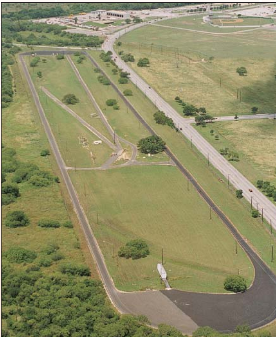
A one-mile track at SwRI is frequently used to provide bumper-to-bumper driveability, endurance, and component evaluation. An eight-mile track is also available for high-speed testing.
