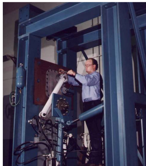
Military Tank Suspension Test Rig
