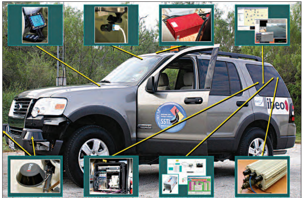
SwRI engineers developed an autonomous vehicle that utilizes enhanced behaviors to traverse roadways with no human in the control loop.
