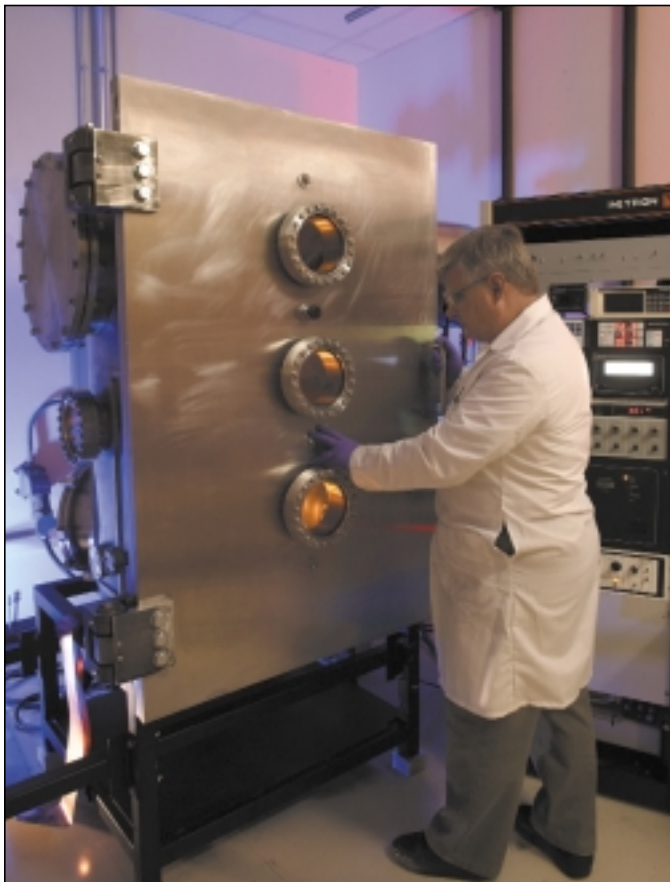
Engineers deposit optical coatings using a state-of-the art cryopumped chamber housed in a dedicated Class 1000 clean room.
