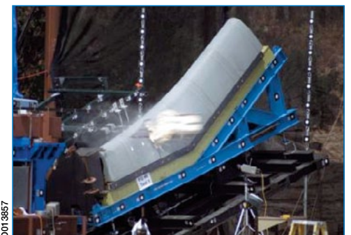
Foam impact test on Space Shuttle wing
