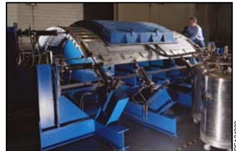
Custom test rigs designed, fabricated and used by SwRI for structural testing
