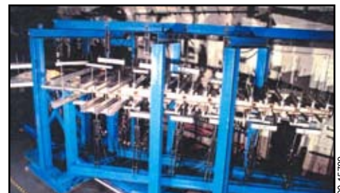
Wing section of T-39 trainer undergoing fatigue testing
